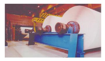
Caledonian Paper decided that the best course of action would be a progressive modernisation programme with the machines selected for the first stage of the programme being the two rewinders which cut the reels of paper to the required diameter and width.
